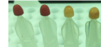
Figure 3. Mitra tips before extraction (left two tips) and after extraction (right two tips). The discoloration of tips indicates successful extraction of whole blood from the tip as a result of the extraction procedure.
